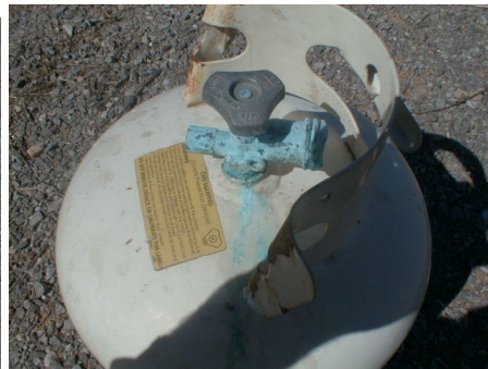
This cylinder has had something other than LP in it and is evident by the discoloration of the valve.
